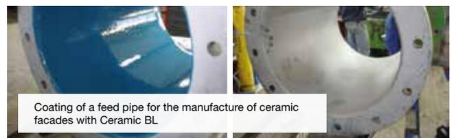
Coating of a feed pipe for the manufacture of ceramic facades with Ceramic BL
