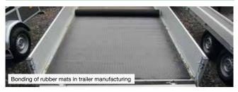
GMK 2410 is an adhesive based on polychloroprene (CR) for the high-strength, full-surface and flexible bonding of
