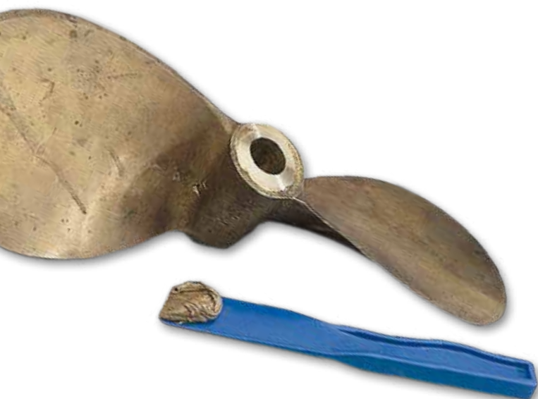
Repair of a ship propeller
