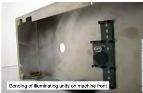
Bonding of illuminating units on machine front
