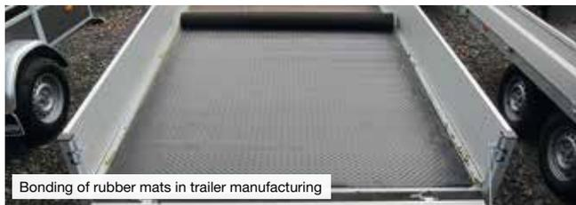
Bonding of rubber mats in trailer manufacturing
